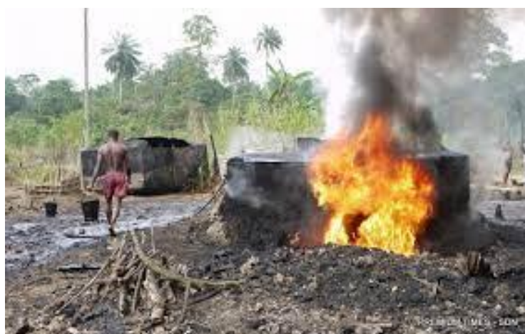
Plate 3: Illegal refinery distillation column
